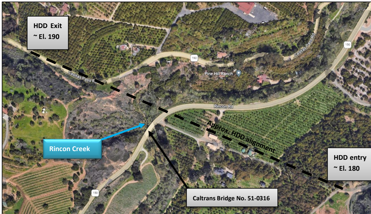
Photo 1 - HDD alignment under Rincon Creek and Rincon Road. See Figures 2 and 3 for Caltrans boring logs at Bridge No. 51-0316.
