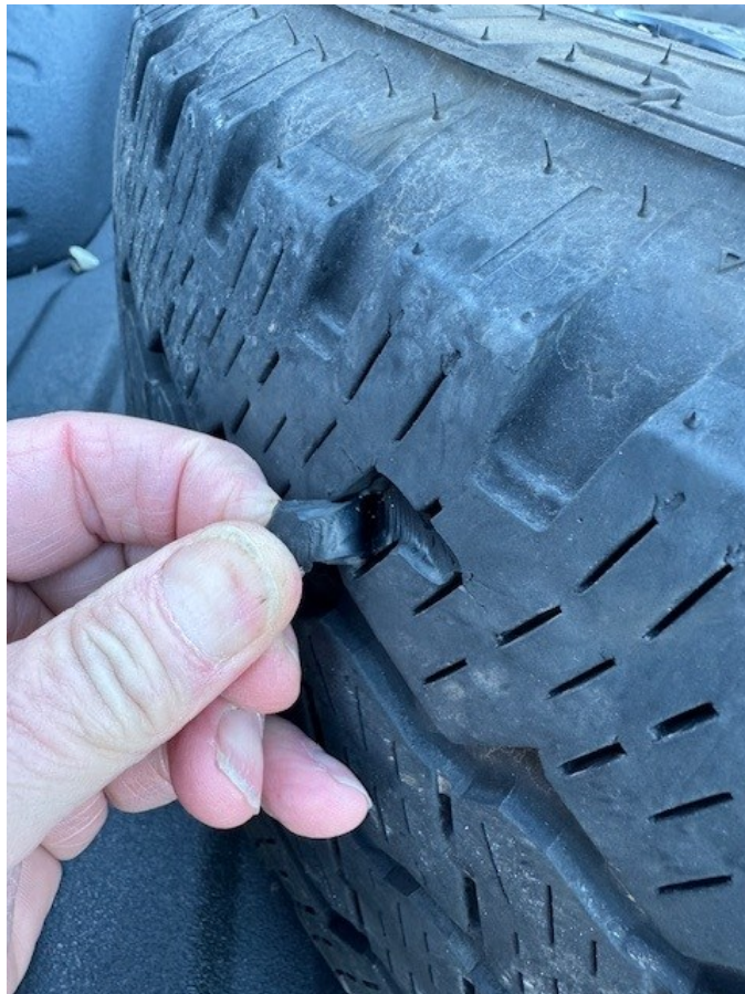
Damage to Tire
